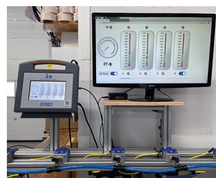
Monitoring system for cleaning nozzles
