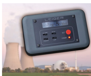
Geiger counter with logging function
