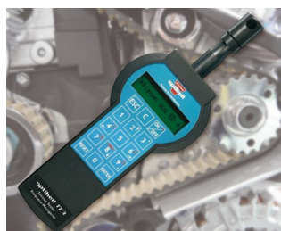
Pretension tester for V-belts and toothed belts
