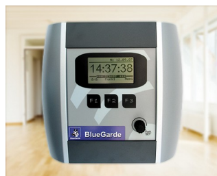
House control unit
