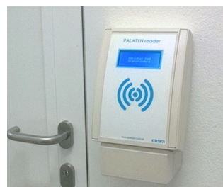
RFID access control readers
