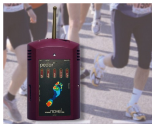
Dynamic pressure measuring between foot and shoe
